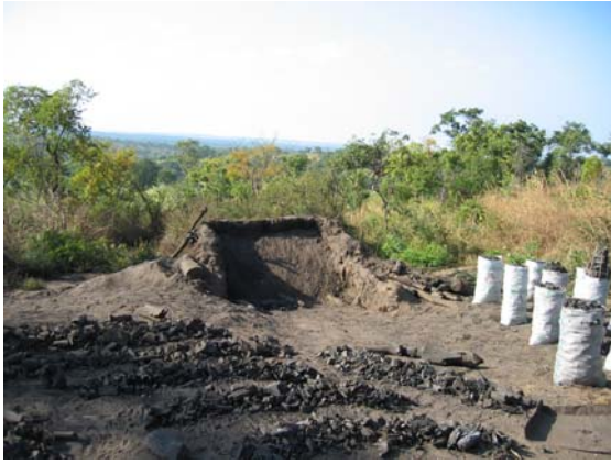
Figure 7 The final step of the production process showing a) a completely burnt kiln at the sorting stage and b) charcoal being unloaded at an estaleiro on the EN-1 in the CR.
