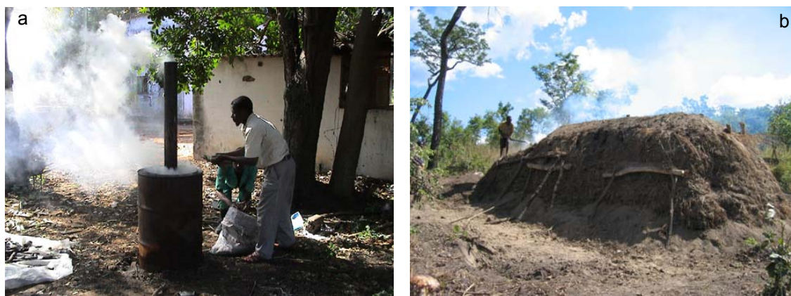
Figure 5 Kiln designs used in Mozambique showing a) an oil drum kiln from the Mucombezi Regulado, Source: UEM (2002) and b) a traditional earth mound kiln from the Chicale Regulado.
